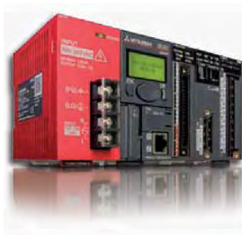
High level, high function modular PLC
